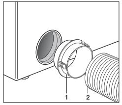
■ Install the exhaust hose/pipe, **2**, with the connector, **1**, to the dryer.
